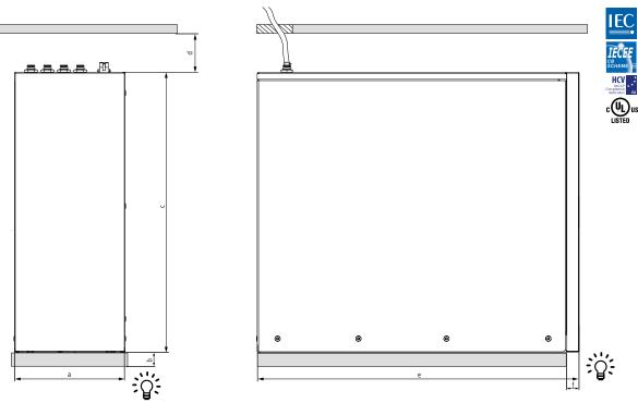
$\dot{\gamma}$  Select the base dimensions so that access to the drawer release is guaranteed.
